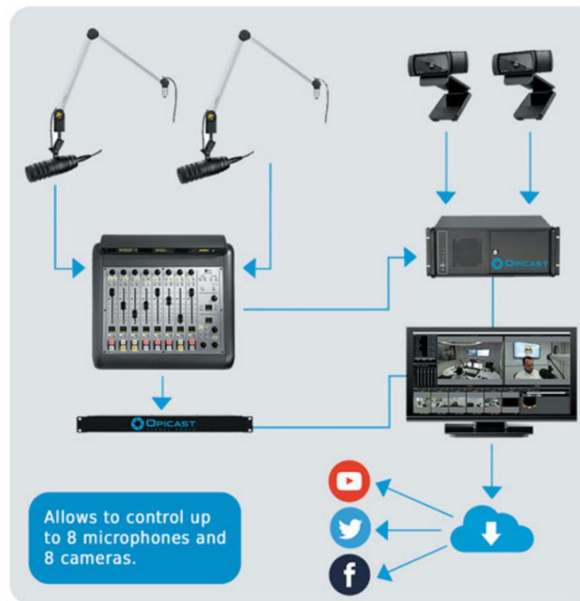
Opicast is an automation solution for radio stations that provides live video streaming of the studio activity. It has a voice detection system, an integrated switcher and an integration/management software. The software can be configured to detect the microphones' activity and cut in the corresponding cameras according to rules created by the user himself.
