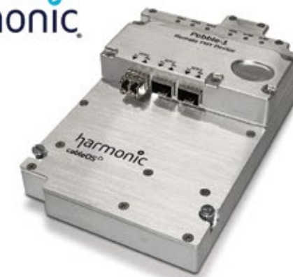
Powered with Harmonic CableOS™ Pebble-1 Remote PHY Device (DOCSIS 3.1 ready)
